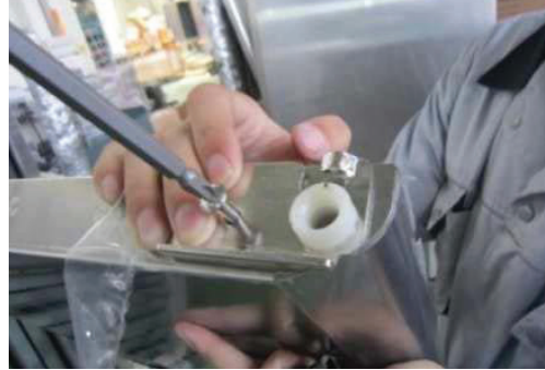
G. Assemble stopper plate in original positions.
