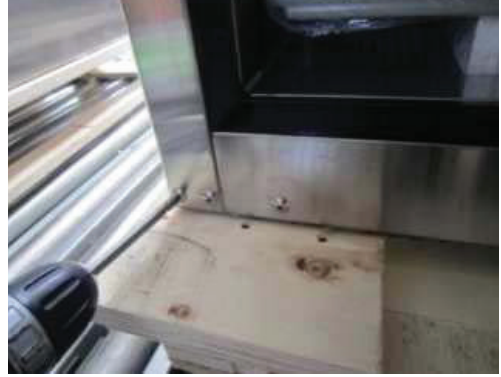
C-2. Disassemble bottom hinge (left).
