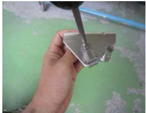
C-2. Disassemble bottom hinge (left).
