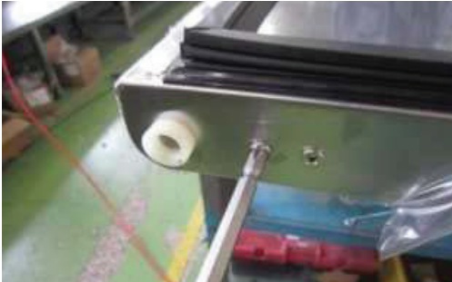
F. Disassemble stopper plate, then tight screws.
