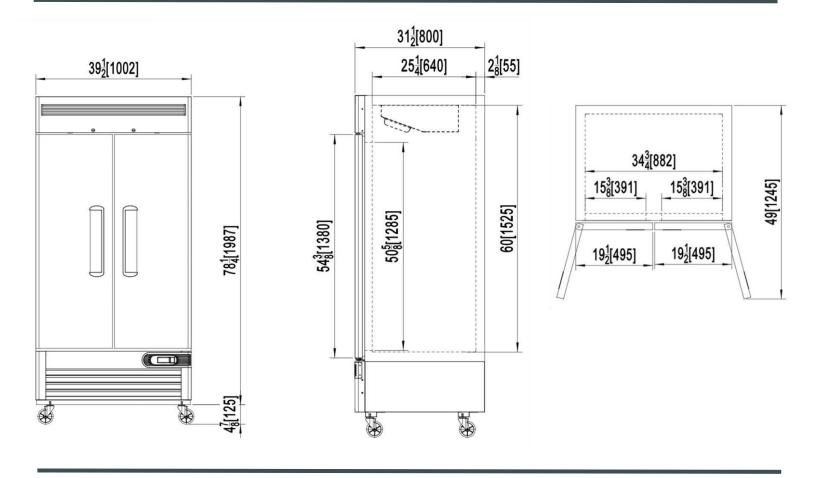
Choose the Frigos Premium FGP-RF-2DBC/40 for a dependable double-door reach-in refrigerator, meeting the demands of commercial kitchens with its generous 30 cubic feet capacity and efficient bottom-mounted compressor. With its emphasis on sustainability, sleek stainless steel design, and easy mobility, this refrigerator ensures both reliability and efficiency for a smoothly operating kitchen.
