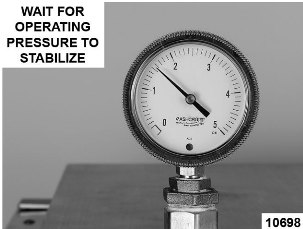
TYPICAL OPERATING PRESSURE
