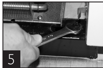
Images 4-6, removing skid from bottom of cabinet.
