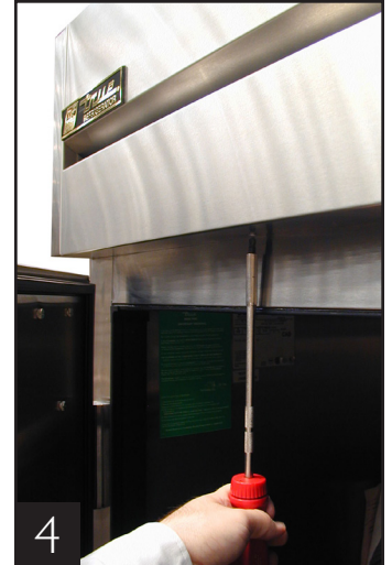
Rainshield removal, bottom screws.
