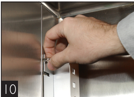
Pilaster installation (side wall of cabinet)
