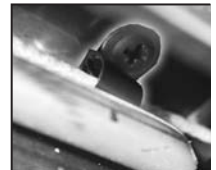
P-Clip keeps cord in-place (prevents cord damage).
