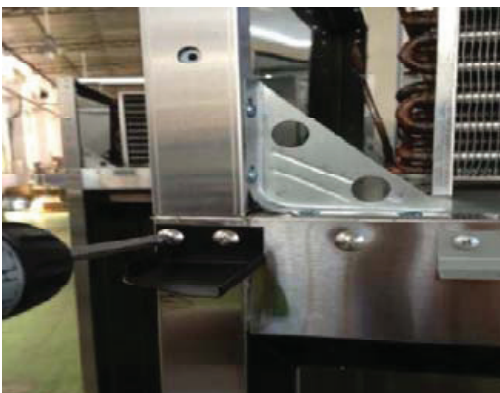
C-1. Disassemble the top hinge (left).
