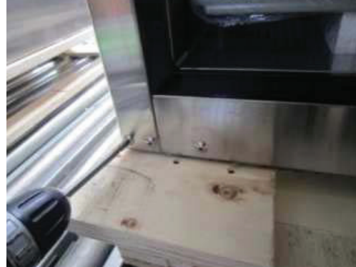
C-2. Disassemble bottom hinge (left).
