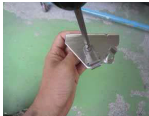
C-2. Disassemble bottom hinge (left).
