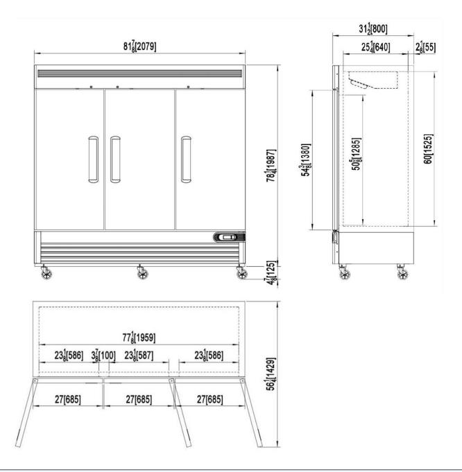
Introducing the Frigos Premium FGP-FZ-3DBC, a top-tier triple-door reach-in freezer with 72 cubic feet of storage. Featuring a bottom-mounted compressor, wide temperature range, and stainless steel construction, it's the ideal solution for efficient and reliable frozen storage in your commercial kitchen.
