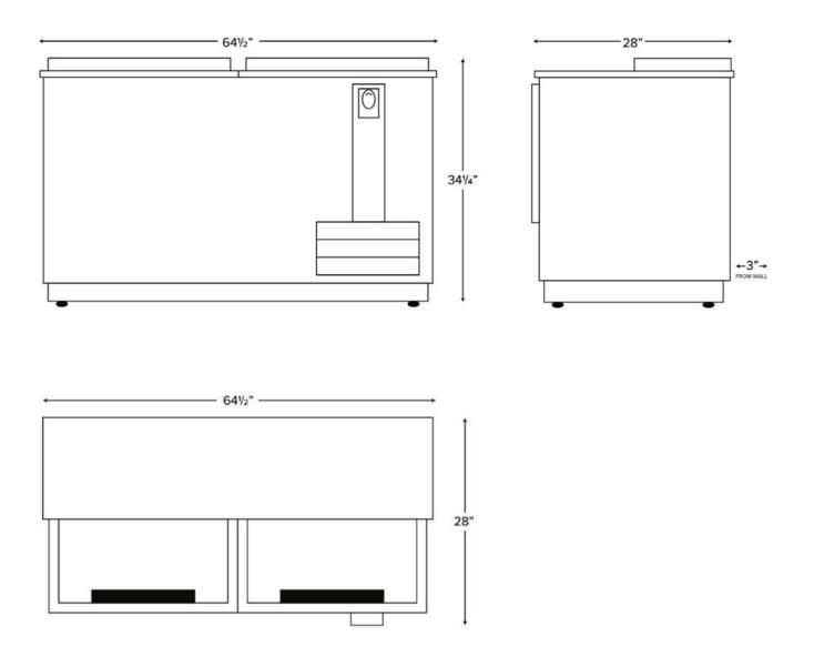
Meet the Frigos Premium FGP-BC-65, a sleek 65" Bottle Cooler with 17.5 cu ft capacity, keeping beverages consistently chilled from 33°F to 41°F. Featuring a stylish black exterior, two sliding lids, and a 1/3+ HP compressor, it brings efficiency and elegance to bars and restaurants. Elevate your beverage service effortlessly with Frigos Premium.
